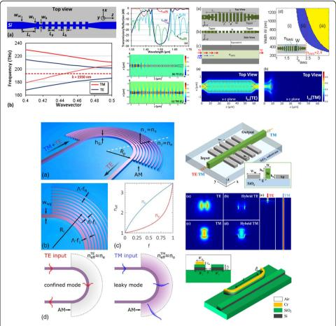
**Fig. 1** Reported on-chip polarizers. **a** An SWG-assisted TM-pass polarizer [28]; **b** An SWG-assisted TE-pass polarizer [26]; **c** A polarizer based on a sharp SWG-assisted waveguide-bend [31]; **d** A polarizer based on an HPWG-assisted grating [37]; **e** A polarizer based on an HPWG-assisted ADC [48]; **f** A TM-Pass polarizer based on a hybrid plasmonic grating [32]
