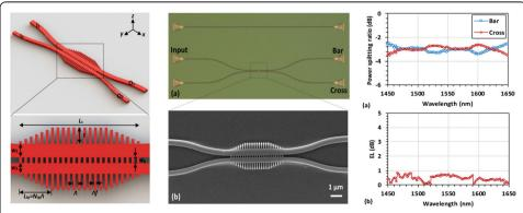
**Fig. 7 a** An ultra-broadband 2×2 3 dB power splitter using an SWG-assisted ADC; **b** SEM image of the fabricated SWG-assisted ADC; Measurement power splitting ratios **c** and ELs **d** for the fabricated SWG-assisted ADC [140]
