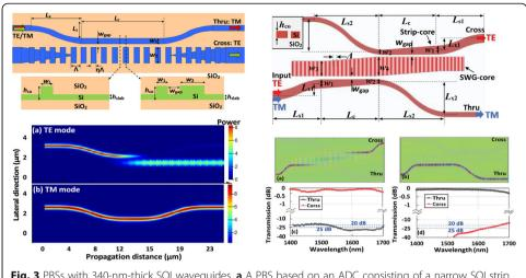
**Fig. 3** PBSs with 340-nm-thick SOI waveguides. **a** A PBS based on an ADC consisting of a narrow SOI strip waveguide and a wide SWG waveguide [65]; **b** A PBS based on SWG-assisted dual-core adiabatic tapers [75]
