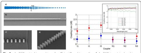
**Fig. 8 a** An SWG-assisted inversed taper for efficient fiber-chip couplings;  $\bf b$  An SWG taper introduced to connect an SOI strip waveguide and an SWG waveguide;  $\bf c$  Measured fiber-chip coupling loss [173]
