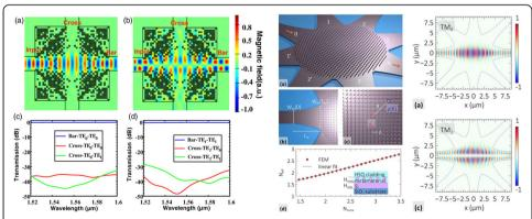
**Fig. 13 a** Dual-mode waveguide crossings based on a subwavelength-structured MMI coupler [248]; **b** A multi-port MWC using a metamaterial Maxwell's fisheye lens [251]
