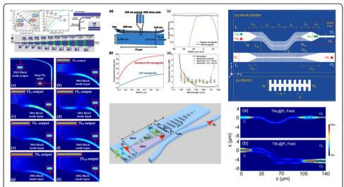
**Fig. 9 a** A 12-channel mode (de) multiplexer based on SWG-assisted ADCs [187]; **b** Higher-order mode (de) multiplexer based on an SWG-assisted dual-core adiabatic tapers [190]; **c** An SWG-assisted multimode add-drop multiplexer [191]; **d** Mode (de) multiplexer based on bridged SWG waveguides [193]
