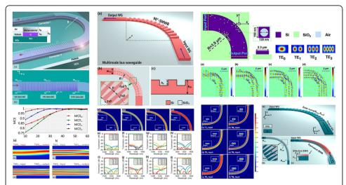
**Fig. 12 a** A sharp MWB with mode converters based on a metamaterial-assisted PMMA upper-cladding [233]; **b** A 90°-MWB based on shallowly-etched non-uniform SWGs [237]; **c** A sharp MWB based on a pixelated meta-structure [238]; **d** A sharp MWB for six dual-polarization modes realized by combining the designs with modified Euler-curve and shallowly-etched non-uniform SWGs [239]
