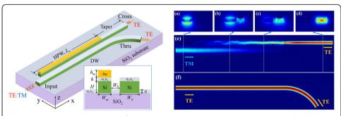
**Fig. 6** A PSR with an ADC consisting of an HPWG and an SOI strip waveguide  $\bf a$ , and the simulated light propagation in the design PSR for the incident TM $_0$   $\bf b$  and TE $_0$   $\bf c$  modes [117]
