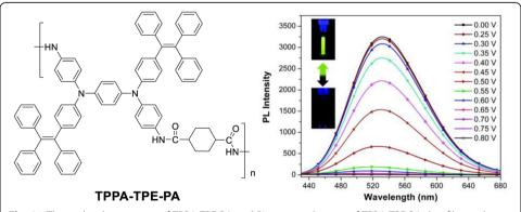
Fig. 21 The molecular structure of TPPA-TPE-PA and PL spectra changes of TPPA-TPE-PA thin film under different voltages. Reprinted with permission from ref. [103] Copyright 2019 Royal Society of Chemistry
