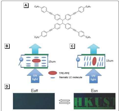
**Fig. 22 a** Chemical structure of TPE-PPE. **b** Electric field-off and **c** field-on (1 KHz, 8 v) states under UV irradiation. **d** Photograph of the LE-LCD device in the electric field-off and field-on states using light-emitting LC mixture. The LC mixture = Nematic LC PA 0182 + 0.1 wt% TPE-PPE. Reproduced with permission from ref. [107]. Copyright 2014 Wiley-VCH
