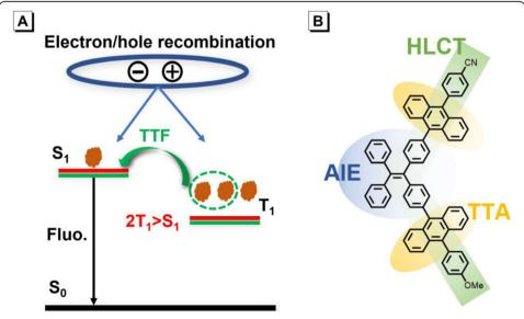
**Fig. 4 a** Typical energy level characteristic of a TTF emitter. **b** Molecule structure of TPEA. Reprinted with permission from ref. [40] Copyright 2018 Royal Society of Chemistry
