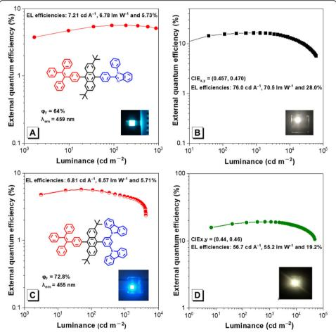
**Fig. 1 a** and **c** EQE – luminance curves of nondoped blue OLEDs for TPE-TAPBI and TPE-TADC; inset: molecule structures, partial photophysical properties, EL properties and device photos; **b** and **d** EQE – luminance curves of WOLEDs for TPE-TAPBI and TPE-TADC; inset: EL properties and device photos. Reprinted with permission from ref. [30] Copyright 2018 Wiley-VCH; and ref. [31] Copyright 2019 American Chemical Society
