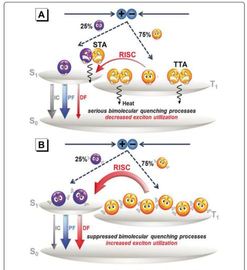
**Fig. 8** The proposed photophysical mechanisms for AIDF molecules in solution and solid state. Reprinted with permission from ref. [58] Copyright 2018 Wiley-VCH
