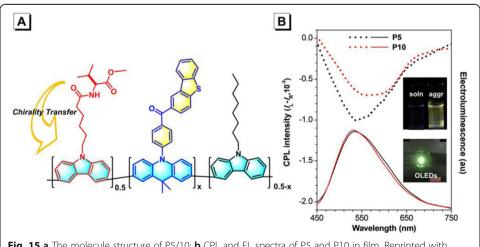
Fig. 15 a The molecule structure of P5/10; b CPL and EL spectra of P5 and P10 in film. Reprinted with permission from ref. [81] Copyright 2019 American Chemical Society
