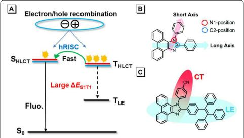
**Fig. 3 a** Typical energy level characteristics of a HLCT emitter with a "hot exciton" channel; **b** the long-short axis design based on phenanthroimidazole. **c** Construction of the LE state and the CT state in *pp*CTPI. Reprinted with permission from ref. [37] Copyright 2019 Royal Society of Chemistry
