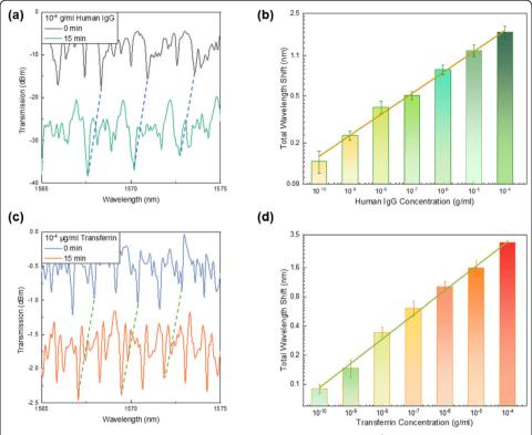
**Fig. 5** WGM laser spectra of the LC-amplified optofluidic resonator under  $10^{-4}$  g/ml (a) human lgG and (c) transferrin at 0 min and 15 mins. The overall wavelength shift responses under different concentrations of (b) human lgG and (d) transferrin
