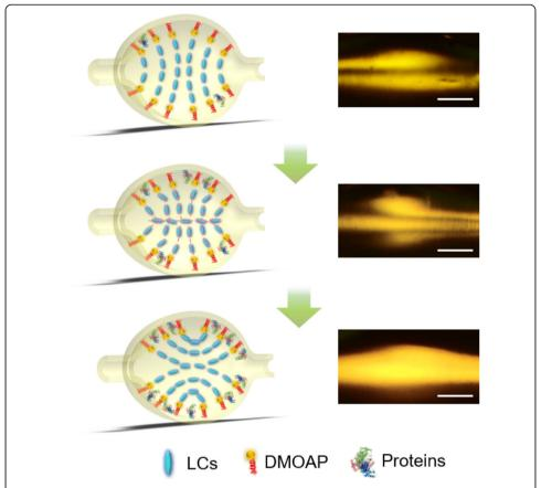
**Fig. 1** Under the disturbance of BSA molecules, the ordering of LC in microcavity is changed. With the increase of BSA concentrations, the illustrations of the ordering of LC molecules gradually changes towards the planer molecular orientation from top to bottom (left). The right panel shows the corresponding polarized optical images of LC-amplified optofluidic cavity. Scale bar:  $100 \, \mu m$
