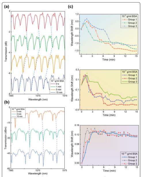
**Fig. 3** WGM laser spectra of the LC-amplified optofluidic resonator under (a)  $10^{-3}$  g/ml BSA (at 0, 1, 5, 15 mins, respectively) and (b)  $10^{-12}$  g/ml BSA (at 0 and 15 mins). (c) Real-time monitoring of WGM laser spectral shift of the LC-amplified optofluidic resonator under different BSA concentrations ( $10^{-3}$ ,  $10^{-7}$ ,  $10^{-12}$  g/ml BSA, from top to bottom) within 15 mins. (Points in the same group are connected by B-spline curve)
