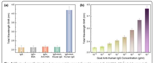
**Fig. 6** Effects of specific binding between anti-human lgG and human lgG. (a) With  $10^{-3}$  g/ml human lgG coated on the silica wall, WGM wavelength shift responses when LCs are exposed to various proteins (BSA, anti-HSA, anti-mouse lgG and anti-human lgG) at the same concentration of  $10^{-3}$  g/ml. (b) WGM spectral shift resulted from antibody-antigen binding events between  $10^{-3}$  g/ml Human lgG and different concentrations of goat anti-human lgG
