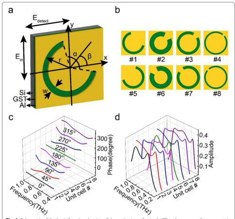
**Fig. 1** Schematic of the basic functional units. **a** Schematic view of a single CR and corresponding geometric parameters.  $\alpha$  is the opening angle, w is the width, r is the outer radius and  $P = 80 \, \mu m$  is the period. **b** Eight CRs unit cell. **c** and **d** simulated phase and amplitude spectra of cross-polarized components of each unit cell
