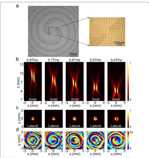
**Fig. 5** Microscopic images and experimental results of fabricated FOV. **a** Microscopic image of fabricated metasurface and the enlarged view of the central area. **b** and **c** Measured normalized intensity distribution of z-x plane and x-y plane at 0.4–0.8 THz. **d** Corresponding phase distribution from **c**
