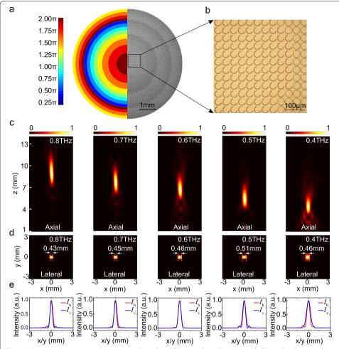
**Fig. 3** Microscopic images and experimental results of fabricated metalens. **a** and **b** Phase distribution of designed metalens and microscopic image of the fabricated metasurface. **c** and **d** Measured normalized intensity distribution of z-x plane and x-y plane at 0.4–0.8 THz. **e** Corresponding extracted far-field normalized intensity profiles of the horizontal (red line) and vertical (blue line) cross-sections from (**d**)
