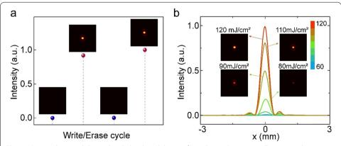
**Fig. 4** Measured repeatability and multi-level modulation of metalens. **a** Experimentally measured normalized intensity distribution for 4 write-erase cycles. **b** Experimentally measured normalized intensity distribution of the horizontal cross-section on the focal plane at varying laser power from 60 to 120 mJ/cm<sup>2</sup> at 10 mJ/cm<sup>2</sup> step
