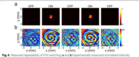
**Fig. 6** Measured repeatability of FOV switching. **a** and **b** Experimentally measured normalized intensity distribution and phase distribution of 5 write-erase cycles
