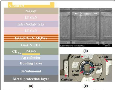
**Fig. 1 a** Schematic of Si-substrate LED vertical structure. **b** SEM image of the top view of the Si-substrate LED with a square contact network. **c** Plan view of the packaged Si-substrate LED. (CE: complementary electrode)
