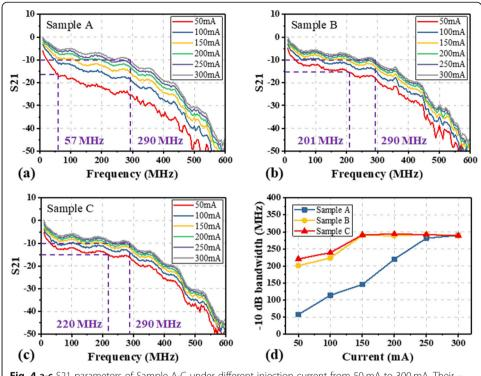
**Fig. 4 a-c** S21 parameters of Sample A-C under different injection current from 50 mA to 300 mA. Their - 10-dB bandwidth values at 50 mA and 300 mA are marked. **d** The - 10-dB bandwidth of three samples under different current
