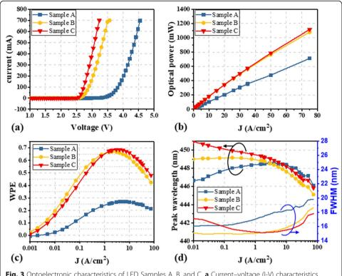
**Fig. 3** Optoelectronic characteristics of LED Samples A, B, and C. **a** Current–voltage (I-V) characteristics under a CW injection current. **b**. Output optical power; **c** Wall-plug efficiency (WPE); **d** Peak wavelength and full width at half maximum (FWHM) of Samples A, B, and C under various current density (J)
