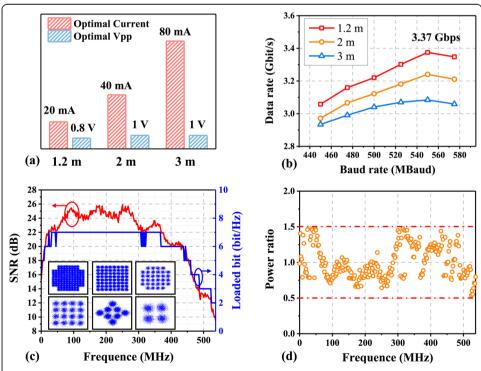
**Fig. 10 a** Optimal current and Vpp for Sample C to obtain the highest SNR. **b** Data rate versus different signal baud rate at the distance of 1.2 m, 2 m and 3 m. **c** SNR and bit distribution at the highest data rate of 3.37 Gbps. Insets: allocated QAM signal diagrams with the loaded bit number from 2 bits/symbol to 7 bits/symbol. **d** Power ratio at each DMT subcarrier after the bit and power loading technology
