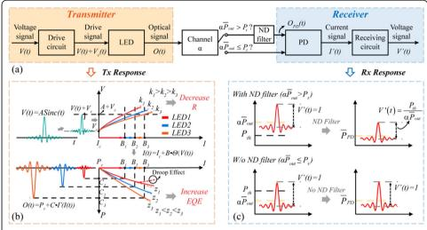
**Fig. 8** Schematic illustration of a VLC system model. **a** Schematic diagram of a typical VLC system. **b** Illustration for the signal response for LEDs with different optoelectronic characteristics. **c** Impact on signal response when the neutral density (ND) filter is applied or not applied. The baud rate of train signal is 550 MBaud
