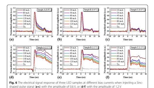
becomes smaller than the small-signal case. Additionally, the SE at the low current range from 10 to 40 mA is lower than that of the small-signal case because the signal with 1.2 Vpp sustains more serious signal clipping at such a low bias current. Once the bias is high enough, signal clipping effect disappears, SE will accordingly rise.
