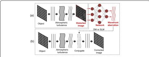
**Fig. 1** Schematic diagram of the deep learning wavefront aberration correction. **a** Production of distortion; **b** wavefront aberration reconstruction and correction
