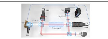
**Fig. 7** Setup for the correction experiment. TL: telecentric lens, CP: calibration plane, ISLM: intensity-type SLM, PSLM: phase-type SLM
