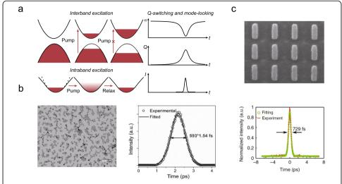
Fig. 6 Meta-optics for laser Q-switching and mode-locking. a Illustration of the processes of saturable absorption based on either interband or intraband excitation (left) and the principle of laser Q-switching and mode-locking (right). b Left: transmission electron micrograph of the ITO nanocrystal. Right: temporal width of one pulse [119]. c Top: SEM image of the plasmonic metasurface. Bottom: temporal width of single soliton [120]
