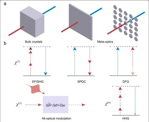
**Fig. 1** Nonlinear optical applications of meta-optics. **a** Schematic comparison of nonlinear optical medium based on conventional bulk crystals and meta-optics. **b** Schematic diagrams of a few representative nonlinear optical processes based on second-, third-, and high-order nonlinear effects that meta-optics may have unique advantages
