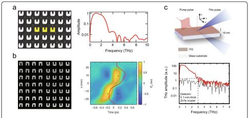
**Fig. 4** Meta-optics for broad THz wave generation. **a** Left: SEM image of the metasurface consists of SRR array. Right: spectrum of the THz wave [99]. **b** Left: SEM image of the metasurface consists of two oppositely oriented SRR array. Right: spatiotemporal profile of the single cycle Hermite Gauss wavepacket [100]. **c** Top: schematic of THz wave generation from an ITO metafilm. Bottom: THz spectrum generated from ITO (red) and the noise spectrum (grey) [45]
