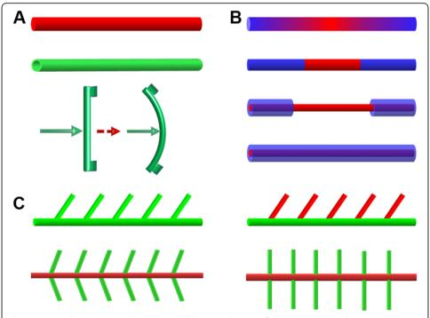
**Fig. 1** Various 1D organic crystal structures. **a** Schematic diagram of 1D organic the single component microcrystals. **b** Schematic illustration of 1D organic multi-component horizontal microcrystals. **c** Graphic expression of 1D organic single/multi-component branched microcrystals
