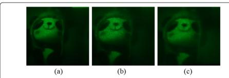
**Fig. 11** Results of the reproduced image when the parameters of the digital conical lens are changed. **a** Result when the reproduction distance is 700 mm; **b** Result when the reproduction distance is 800 mm; **c** Result when the reproduction distance is 900 mm
