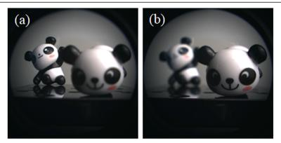
**Fig. 14** Results of the captured images when only one liquid lens is actuated. **a** Applied voltage U = 36 V; **b** applied voltage U = 55 V
