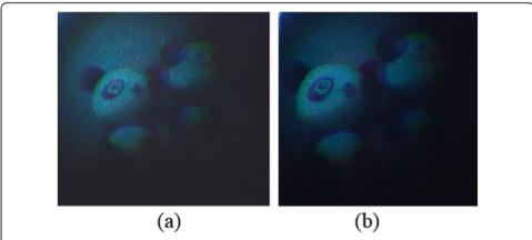
**Fig. 13** Results of the reproduced images when the focal length of the zoom camera changes. **a** Reconstructed image when F = 26.08 mm; **b** reconstructed image when F = 31.87 mm
