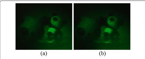
**Fig. 15** Reconstructed images when only one liquid lens is actuated. **a** Applied voltage U = 36 V; **b** applied voltage U = 55 V
