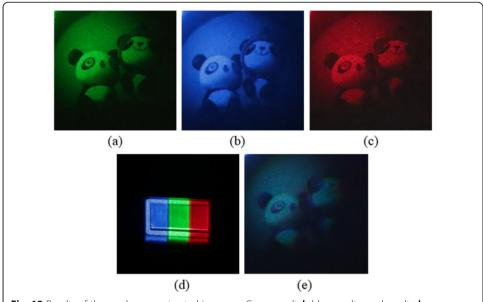
**Fig. 12** Results of three color-reconstructed images. **a** Green result; **b** blue result; **c** red result; **d** experimental diagram of the SLM; **e** color result
