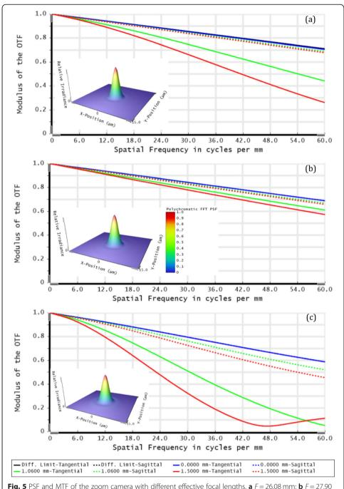
**Fig. 5** PSF and MTF of the zoom camera with different effective focal lengths. **a** F = 26.08 mm; **b** F = 27.90 mm; **c** F = 32.26 mm
