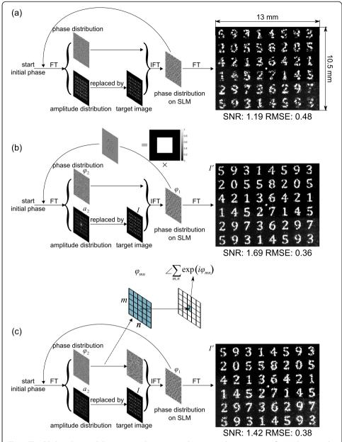
**Fig. 2** The GS algorithms and the corresponding generated images in the experiments for (a) the original GS algorithm (worst);  $\bf b$  constraining the phase distribution in SLM plane with a window (best);  $\bf c$  modifying the variation of the phase distribution in image plane (good)
