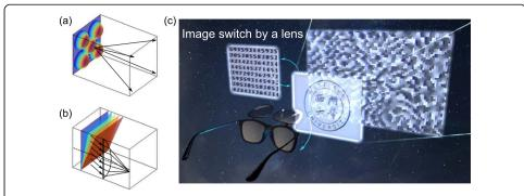
**Fig. 1 a** and **b** The interpretation of light as a superposition of spherical waves and plane waves.  $\bf c$  Example application of the holographic displays multiplexed by a lens
