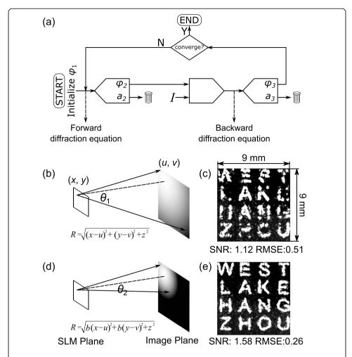
**Fig. 3 a** The GS algorithm employing the RS diffraction equations. **b** and **d** The amplitude distributions on the image plane calculated by the unmodified and modified forward diffraction equations, respectively. **c** and **e** The images generated by the GS algorithms with the unmodified and modified forward diffraction equations, respectively
