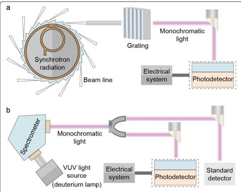
**Fig. 3** Test method for photoelectric response characteristics of VUV photodetectors. **a** The test is carried out by the line station of synchrotron radiation vacuum ultraviolet light source. **b** The test is carried out by a test system built with VUV light sources such as deuterium lamps and standard detectors as the radiation transfer standard
