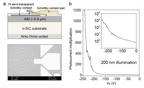
**Fig. 9** Structure and performance of AIN-based avalanche VUV photodetector. **a** Schematic layer structure and SEM image of a fabricated AIN avalanche photodetector with  $d=100\,\mu m$  in diameter. **b** Photocurrent multiplication or gain of an AIN avalanche photodetector as a function of the reverse bias voltage. The inset is as same as the semilog scale [126, 127]
