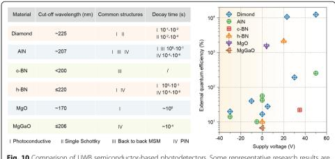
**Fig. 10** Comparison of UWB semiconductor-based photodetectors. Some representative research results are enumerated in the right figure
