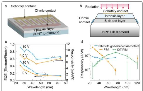
**Fig. 5** Structure and performance of Schottky VUV photodiodes. **a** Schematic drawing of the interdigitated-finger Schottky photodiode based on p-diamond epilayer [81]. **b** Structure of the p-type/intrinsic/metal (PIM) device [82]. **c** The responsivity and the EQE of the PIM device measured at two different values of the applied bias from 20 nm to 80 nm [82]. **d** Responsivity of the PIM and IDT-PIM (with interdigitated finger electrodes) diamond detectors [83]
