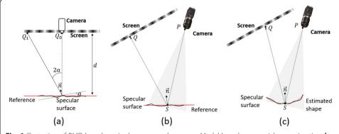
**Fig. 1** Illustration of PMD based on single screen and sensor. **a** Model based on paraxial approximation; **b** model based on flat reference; **c** model based on an estimated shape and position of SUT
