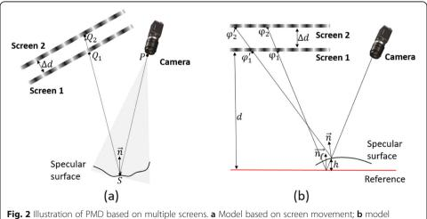
Fig. 2 Illustration of PMD based on multiple screens. a Model based on screen movement; b mode of DPMD
