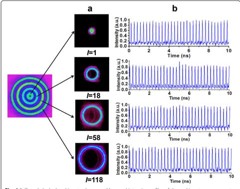
**Fig. 4** Self-mode-locked multi-vortex beams. **a** Measured intensity profiles of the multi-vortex components. **b** Measured pulse trains of the multi-vortex components
