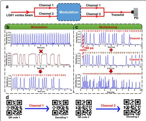
**Fig. 6** Temporal encoding and time-division multiplexing (TDM) of pulsed vortex beams for data transmission. **a** Schematic of TDM of the pulsed LG<sub>01</sub> vortex beam. **b** Temporal encoding of one divided pulsed vortex beam. **c** Multiplexing of two encoded pulsed vortex beams. **d** Measured data transmission results for two QR codes transfer using temporal encoding and TDM of pulsed vortex beams
