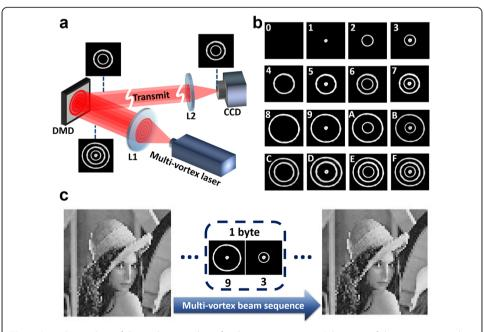
**Fig. 5** Spatial encoding of the multi-vortex laser for data transmission. **a** Schematic of data transmission by spatial encoding of the multi-vortex laser. DMD: digital micromirror device. **b** Measured patterns of the multi-vortex laser encoded by DMD and the corresponding hexadecimal codes. **c** Measured data transmission results for image transfer using spatial encoding of the multi-vortex laser
