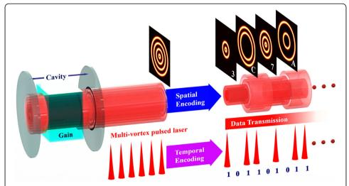
**Fig. 1** Concept and principle. Multi-vortex pulsed beams are generated directly from the laser. Spatial encoding is achieved by combining specific components of the vortex beams, and temporal encoding is achieved by modulating the pulses. Both spatial and temporal encoding are used for data transmission
