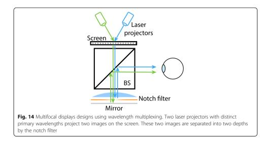
focal planes by wavelength multiplexing, there are still many challenges for practical applications. Firstly, mixing wavelengths in each color channel would directly affect the overall color performance, since only colors shared by all focal planes can be displayed if a uniform system color appearance is desired. Also, the stopband of the notch filter usually shifts under different angles of incidence, which becomes a critical limitation for achieving a larger FOV.
