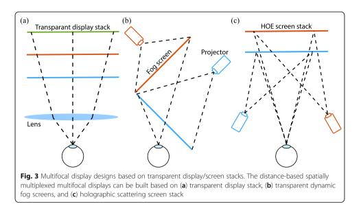
pixels in cascaded panels, the Moiré effect [41] may happen through the multiple panels. The resulting Moiré fringes would degrade the quality and resolution of displayed images.
