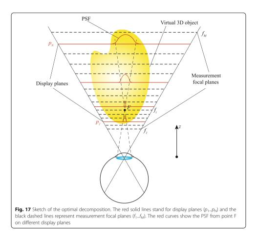
weights. Therefore, the space is segmented into M measurement focal planes to evaluate the rendering in different depths.
