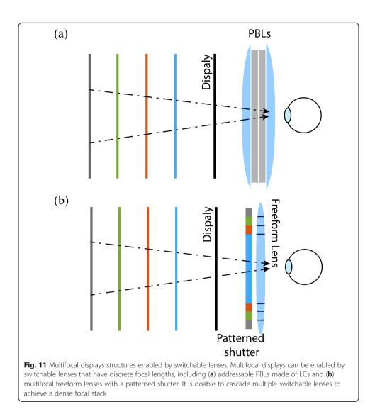
switching between focal planes using continuously tunable lenses. A general limitation of this design and others using switchable lenses is that it cannot realize the dynamic multifocal structure proposed by Wu et al. [91] because of the fixed focal plane arrangement.
