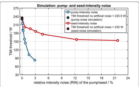
**Fig. 8** Simulation results of the dependence of the TMI threshold on the relative intensity noise (RIN) of the pump (blue circles) and the seed (red circles). The simulations are in good agreement with the experimental results (Fig. 7)
