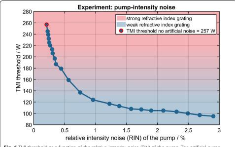
**Fig. 6** TMI threshold as a function of the relative intensity noise (RIN) of the pump. The artificial pump intensity-noise contains frequencies from 1 Hz up to 2 kHz. For a value of 2.9% the pump-RIN decreases the TMI threshold by 63% from its intrinsic value (95 W vs. 257 W)
