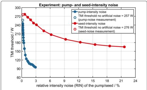
**Fig. 7** TMI threshold as a function of the relative intensity noise (RIN) of the pump and the seed. The artificially imprinted noise contains frequencies from 1 Hz up to 2 kHz. The impact of the pump intensitynoise (blue dots) on the TMI threshold is significantly stronger than that of the seed intensity-noise (red dots)
