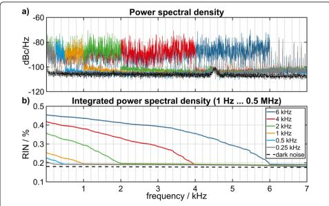
**Fig. 2** Measured pump intensity-noise with different cut-off frequencies. **a** Power spectral density and **b** Relative intensity noise (RIN: integrated power spectral density from 500 kHz down to 1 Hz; the frequency range for the integration is determined by the sample rate of the oscilloscope and by the acquisition time)
