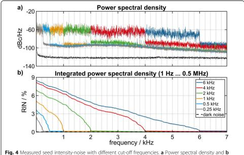
**Fig. 4** Measured seed intensity-noise with different cut-off frequencies. **a** Power spectral density and **b** Relative intensity noise (RIN: integrated power spectral density from 500 kHz down to 1 Hz; the frequency range for the integration is determined by the sample rate of the oscilloscope and by the acquisition time)
