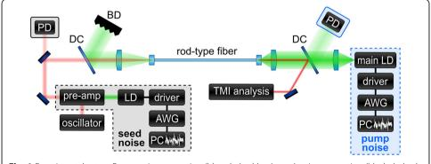
**Fig. 1** Experimental setup. Pump-noise generation (blue dashed box), seed-noise generation (black dashed box), pump-noise measurement (blue solid box), seed-noise measurement (black solid box); AWG - arbitrary waveform generator, BD - beam dump, DC - dichroic mirror, LD - laser diode, PC - personal computer, PD - photodiode
